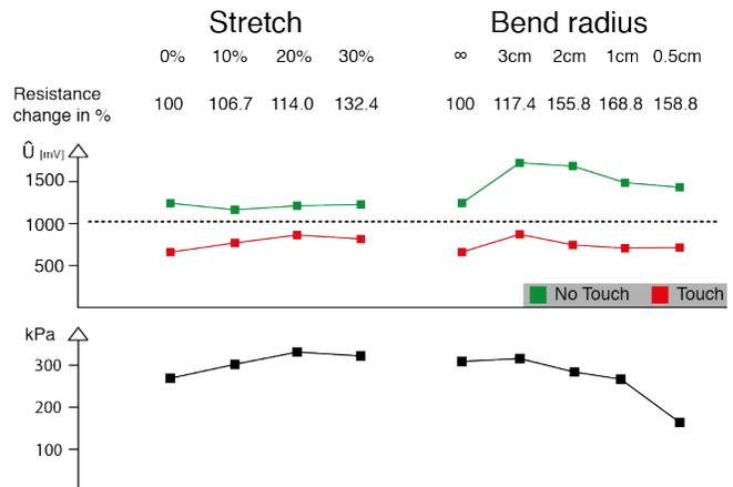
**Figure 4. Results of the technical evaluation:** (a) relative change in resistance, (b) measured voltage  $\hat{U}$  for capacitive touch contact and no touch, (c) required pressure for resistive touch contact.
