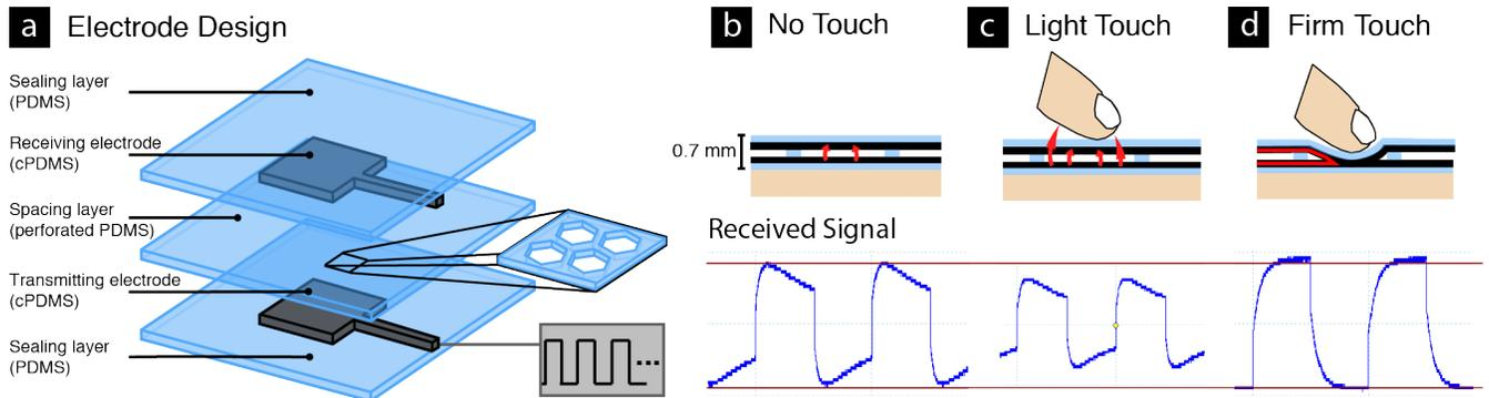
**Figure 2. iSkin Touch Sensing:** (a) Overview of layers in a touch-sensitive iSkin; (b) sensing without touch contact; (c) projected capacitive sensing of slight touch events; (d) resistive sensing of firm touch events.
