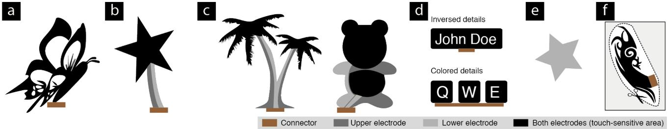
**Figure 3. Design Patterns for Visual Customizations:** (a) fully touch-sensitive graphic, (b) partially sensitive graphic, (c) graphic with multiple interactive areas, (d) touch-sensitive detail using inverse and color patterns, (e) non-sensitive visual elements, and (f) shape customization.
